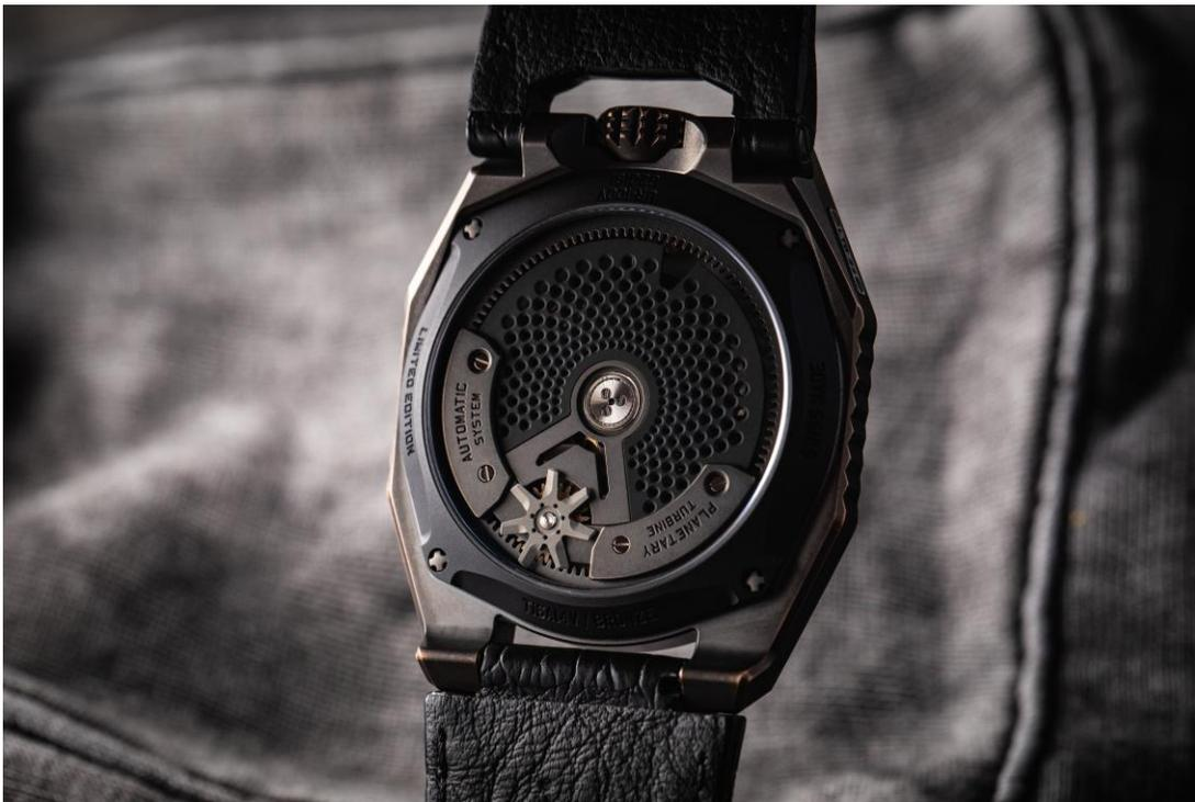
The regular orbit of the hours, as old as time itself, replicates the planetary dance in miniature. The watch is wound while you wear it by a rotor. This is coupled to a device called the Windfänger that is specific to the UR-100 models. It's a planetary gear that limits the action of the rotor to avoid overwinding and excessive wear.
