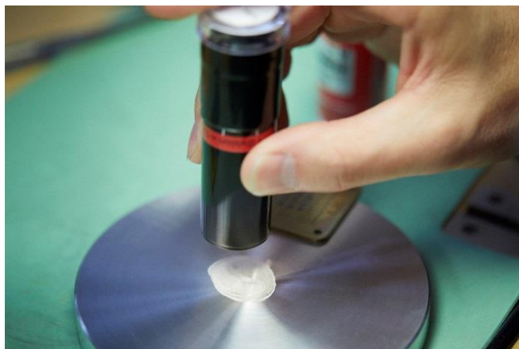
The screws are screwed into a holder while diamond polishing paste is prepared on a tin plate. The heads of the screws are ground flat and polished to a mirror finish.
