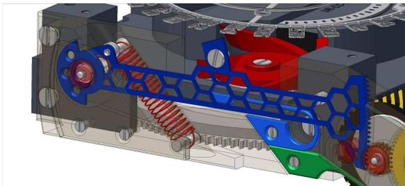
The energy released by the retrograde mechanism is recovered and used to power the rotation of the jumping hour cylinder. Visible through a display panel in the side of the case, a 12 pointed star and positioning spring are the only distinguishable components of this innovative mechanism for recycling energy
