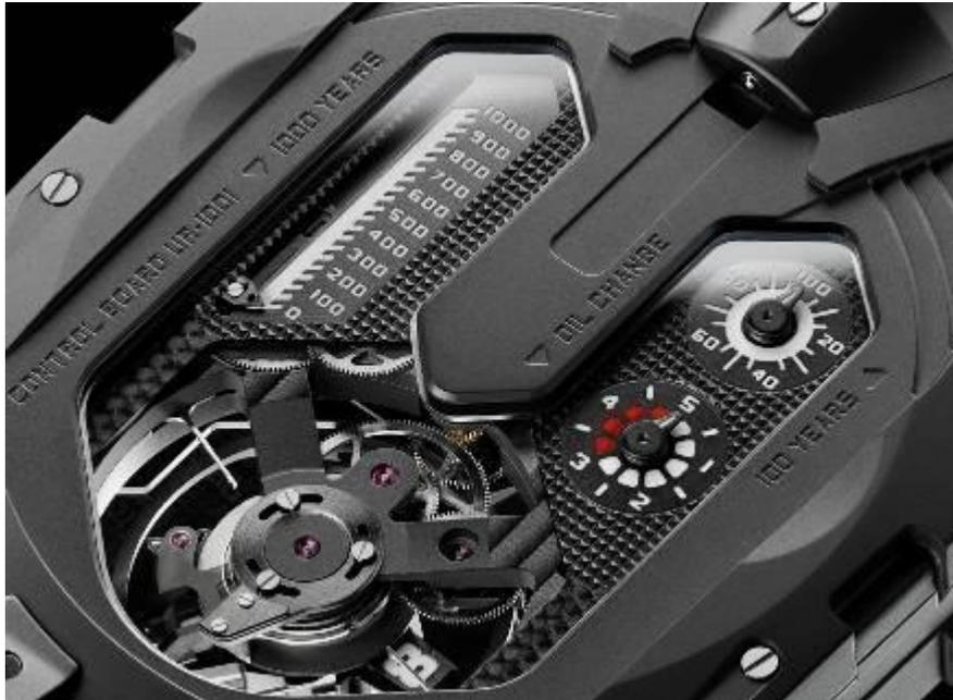
**“Oil Change” indicator.** The shortest time interval measured on the back is the 5-year “Oil Change” indicator at centre right, which alerts the user when a service is due after three years when the dial changes from white (years one to three) to red (years three to five). This counter is reset to zero when the timepiece is serviced.
