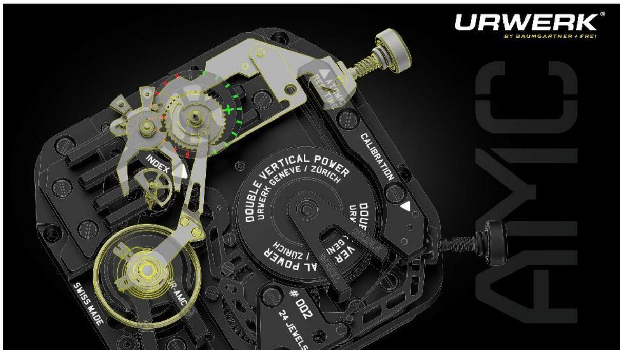
The rate of a watch is controlled by the regulator. The regulator usually takes the form of a so-called index, which controls the effective length of the balance spring. If a watch is found by the owner to be running too fast or too slow, the index can be moved to adjust the effective length of the balance spring, to essentially speed up or slow down the rate of the watch.
